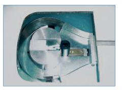
Semi automatic shirt folding table with automatic collar opening according to the size. Electrically heated collar shape. Rack for carton, pins holding. Productivity 30-40 pcs/h - Electric connection 230V-1Ph-50Hz - Compressed air 5 bar
